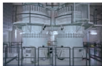
反応科学超高压走査透過電子顕微鏡 JEM1000K RS Reaction science high voltage scanning transmission electron microscope (JEM 1000K RS)
