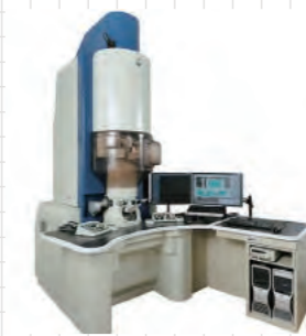
高分解能電子状態計測走査透過電子顕微鏡 JEM-ARM200 (Cold) (収差補正電子顕微鏡) Aberration corrected scanning TEM JEM ARM200F
