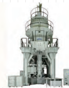
反応科学超高压走査透過電子顕微鏡 JEM 1000K RS Reaction science high voltage scanning TEM JEM1000K RS
