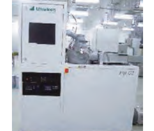
ALD(プラズマ式/サーマル式) UltraTech/CambridgeNanoTech Fujii G2 Atomic layer deposition system (Plasma/Thermal) UltraTech/CambridgeNanoTech Fujii G2
