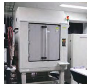
エミッション顕微鏡 HAMAMATSU PHOTONICS PHEMOS-1000 Emission microscope HAMAMATSU PHOTONICS PHEMOS-1000
