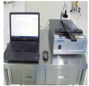
光干渉膜厚計(自動マッピング式) FILMETRICS F50 Automated Thickness Mapping Systems FILMETRICS F50
