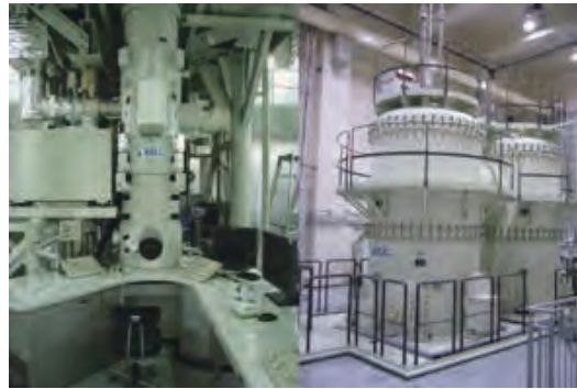
反応科学超高圧走査透過電子顕微鏡 JEM1000K RS Reaction science high voltage scanning transmission electron microscope (JEM 1000K RS)
