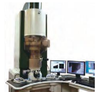
電界放出型走査透過電子顕微鏡 JEM-10000BU (収差補正電子顕微鏡) Aberration corrected scanning TEM JEM-10000BU
