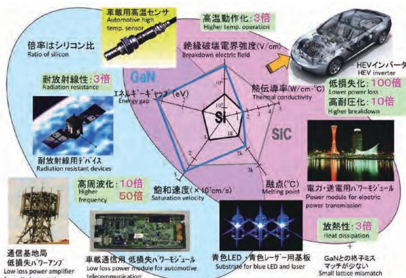
次世代パワー半導体の特長と応用 Characteristics and applications of next-generation power semiconductor
