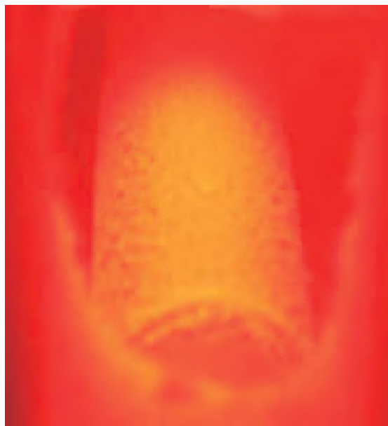
灰附着炉内での伝熱管試料表面への灰附着状況 Picture of heat exchanger tube in vertical ash deposition furnace
