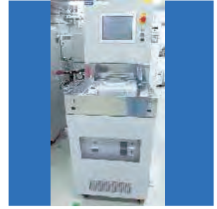
P-CVD1 samco PD-220NL Plasma CVD 1 samco PD-220NL
