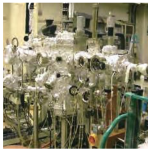
8元MBE装置 MBE with 8 sources
