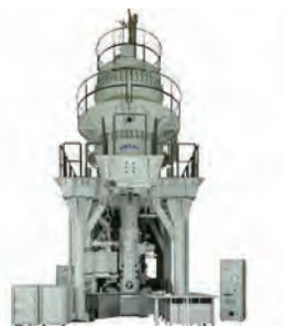
反科学超高压走査透過電子顕微鏡 JEM 1000K RS Reaction science high voltage scanning TEM JEM1000K RS
