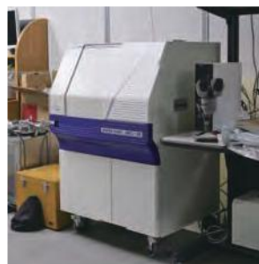
仕事関数測定装置 RIKEN KENKI AC-3 Work function measuring device RIKEN KENKI AC-3
