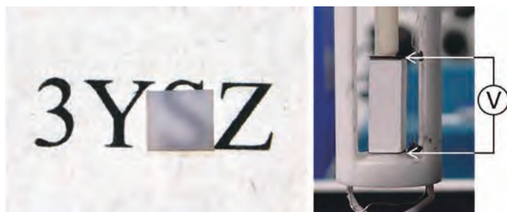
3mol%Y 2 O 3 -ZrO 2 ceramic by HAfS flashing technique at 1200°C for only 5min.
